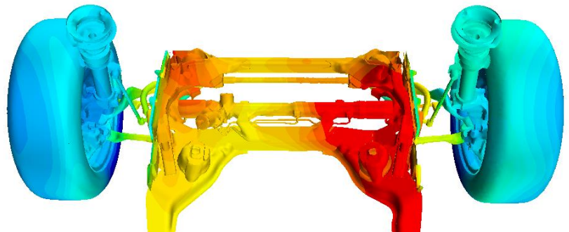
Temperature distribution of the front axle including engine mounting and steering gear
