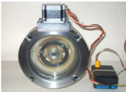
**Figure 2** Planetary gearbox driven by stepping motor.
