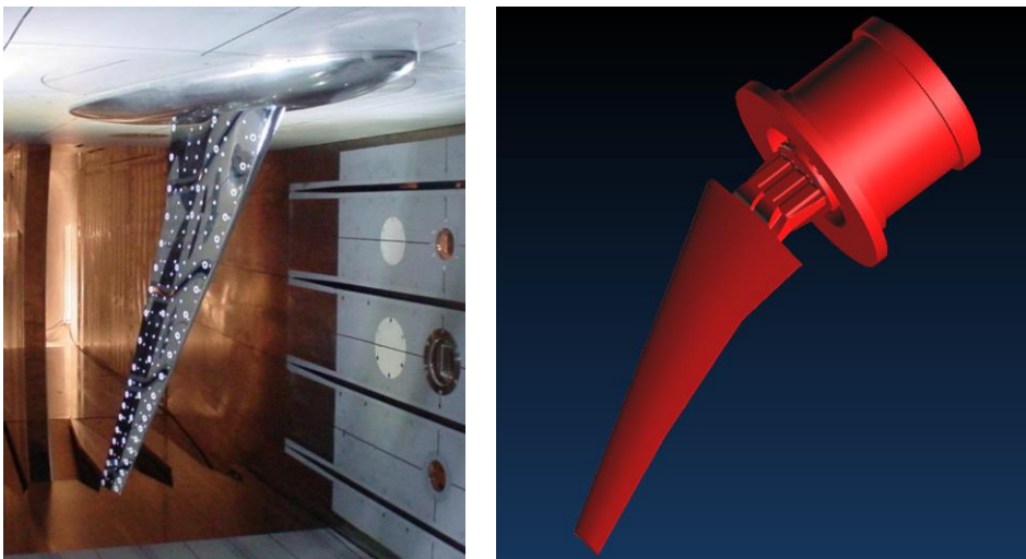
Figure 2: Hirenasd wind tunnel assembly on the left, and FEA model of the wing and excitation model on the right.
